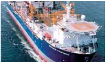
Ship name: Deepwater pathfinder Owner: Conoco/R&B Falcon Type: Dynamically-positioned drillship Design: R&B/Conoco - double hull Yard: Samsung Heavy Industries, Korea
