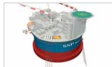
Ship name: Sevan "SSP 300 for Chestnut" Owner: Sevan Marine ASA Type: FPSO - Floating Production, Storage and Offloading Design: SSP 300 Yard: Yantai Raffles Yard, China
