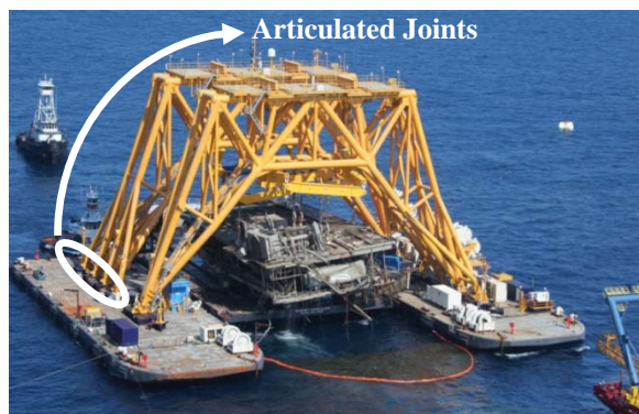
Fig. 2 Bottom Feeder System in Operation Using Pin-in-Pin Articulated Joints
