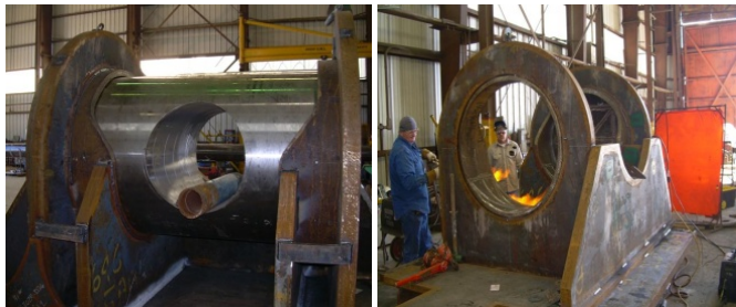
Fig. 1 Fabrication of Pin-in-Pin Articulated Joint
