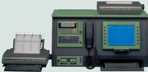
This solution is used for Sea Area A3 and occasionally for Sea Area A4. The picture shows a two-section console containing a SAILOR HC4500 MF/HF controller, a SAILOR H2095C SAT-C transceiver unit, battery panel, loudspeaker, emergency light and SAILOR DT4646E data terminal. The SAILOR H1252B printer on the console is fed paper from a roll in the console, which also contains the connection board. Next to the console are the keyboard and the radio telex printer for GMDSS radio telex operation.
