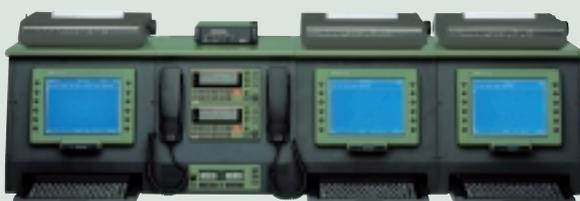
The SAILOR dual radio telex solution with optional Sat-C for Sea Area A4 is shown here in a four-section console containing 2 x SAILOR HC4500 MF/HF control units, SAILOR H2095C SAT-C transceiver, battery panel, loudspeaker, emergency light, 3 x SAILOR DT4646E Dataterminals with keyboards and printers. Printer paper is fed from a role in the console, which also contains the connection board.
