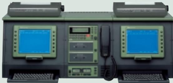
The SAILOR GMDSS dual SAT-C solution for Sea Area A3 is shown here in a three-section console containing a SAILOR HC4500 MF/HF controller, 2 x SAILOR H2095C SAT-C transceiver units, battery panel, loudspeaker, emergency light, 2 x SAILOR DT4646E with keyboards and printers. Printer paper is fed from a role in the console, which also contains the connection board.
