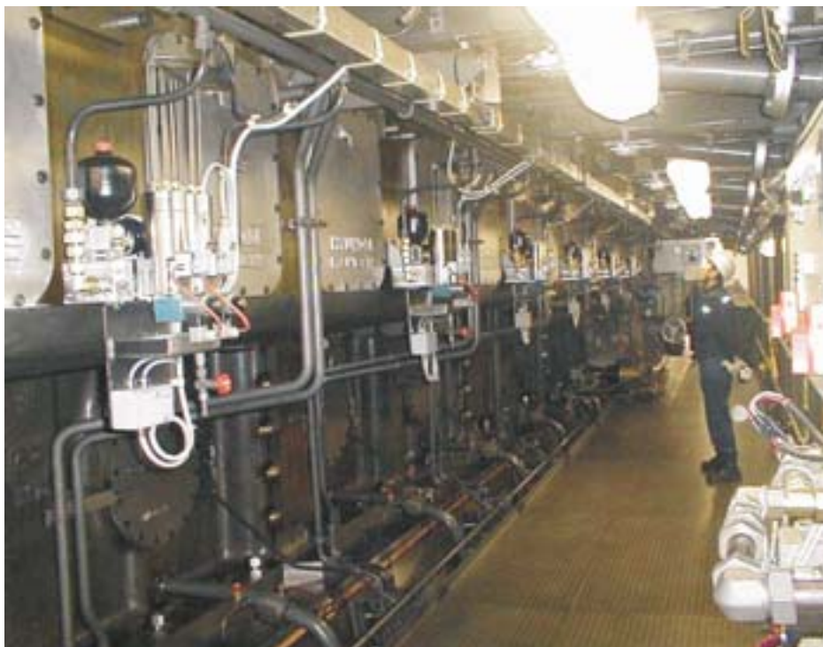
Fig. 1: Alpha Lubricator fitted on a 12K98MC-C main diesel engine
