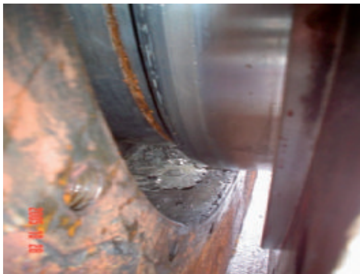
Fig. 1: Pieces of white metal found in the aft stern tube bearing after removal of seal.
