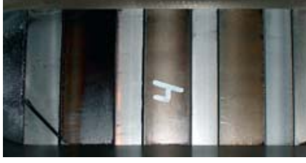
Fig. 8. Unit running very well after 20,021 running hours. Note that the last remains of the alu-coat are still visible on the lower edge, indicating remaining rounding left. This means that the ring wear is less than 2 mm out of possible 3 mm. Consequently, many more hours are left from the point of view of wear.
