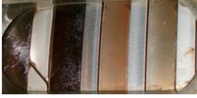
Fig. 5. Unit with 23,500 hours without piston overhaul. Note that most of the rounding is still intact, indicating that only \frac{1}{4} of the wear potential is used. Further, the measurements above from the same unit shows that only \frac{1}{2} of the ring groove wear potential is used, and the rate of burnings on the piston top is insignificant. Consequently, overhaul of that unit is not needed at this stage.
