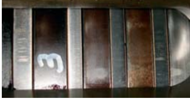
Fig. 7. Unit with micro-seizures on the top and bottom rings as a result of metal-to-metal contact. Should be counteracted by temporarily increased lubrication. It is important to lower the lubrication to normal as soon as the active mz-attack is stopped. Note that old, not active, mz-marks remain visible a long time and do not call for increased lubrication.
