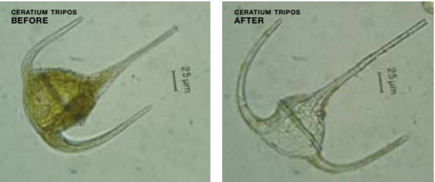
Radicals produced within the PureBallast system disrupt the cell membrane of microorganisms, such as the dinoflagellate pictured here. After passing through a Wallenius AOT unit, the dinoflagellate has lost its chlorophyll, making it unable to reproduce.
