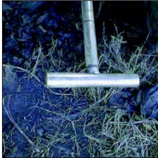
Figure 11 T-bar penetrometer
