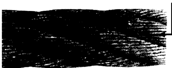
FLAT SURFACE DUE TO WEAR
