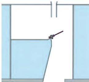
Open joint with drainage
