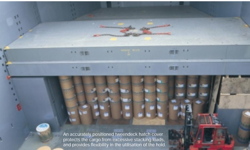
An accurately positioned tweendeck hatch cover protects the cargo from excessive stacking loads, and provides flexibility in the utilisation of the hold.
