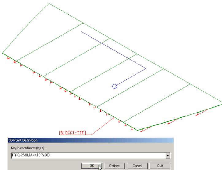
The purpose of this program is to define co-ordinates and planes that later can be referred to in the Tribon Outfit modelling systems. So, for example, one can then refer to waterlines, decks etc instead of always using absolute co-ordinates (distances from the ships origin where  $x=0, y=0, z=0$ ).
