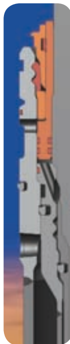
SHD Rigid Lock Seal Assembly Interface with Low and High Pressure Housing
