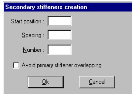
Figure 14 : SECONDARY STIFFENERS CREATION WINDOW
