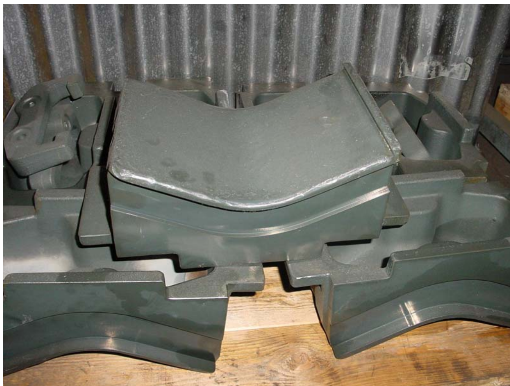
FIG. 2-2 Set for external diameter (fixed saddles)
