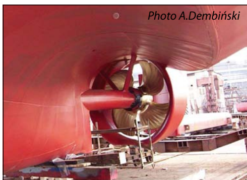
4. Ducted propeller
