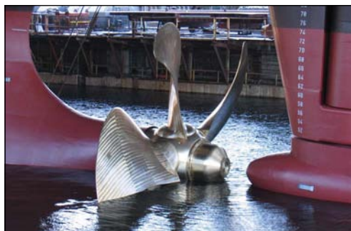
1. Adjustable bolted propeller
