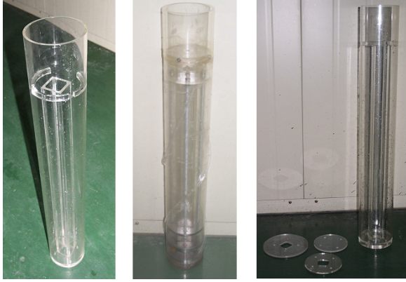
Fig. 2 Model configurations : model with moonpool, strakes, and damping plates
