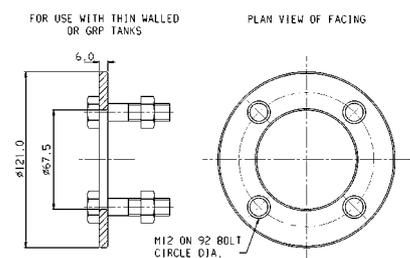
J184 in 316SS: 71020/107 (Not suitable with Mobrey 'M' switch SMA\*)
