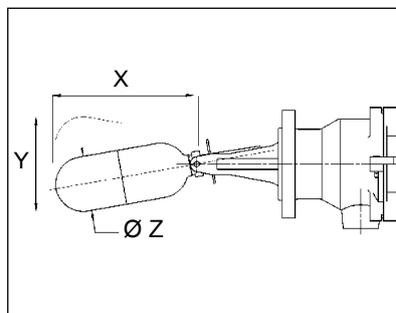
This is the most popular switch in the Mobrey range. Its size and robust construction make it ideal for a wide range of general purpose and industrial applications such as pump control and high or low level alarm on tanks and pressure vessels. The dimensions for the float in the diagram left can be found on fold out page 22.
