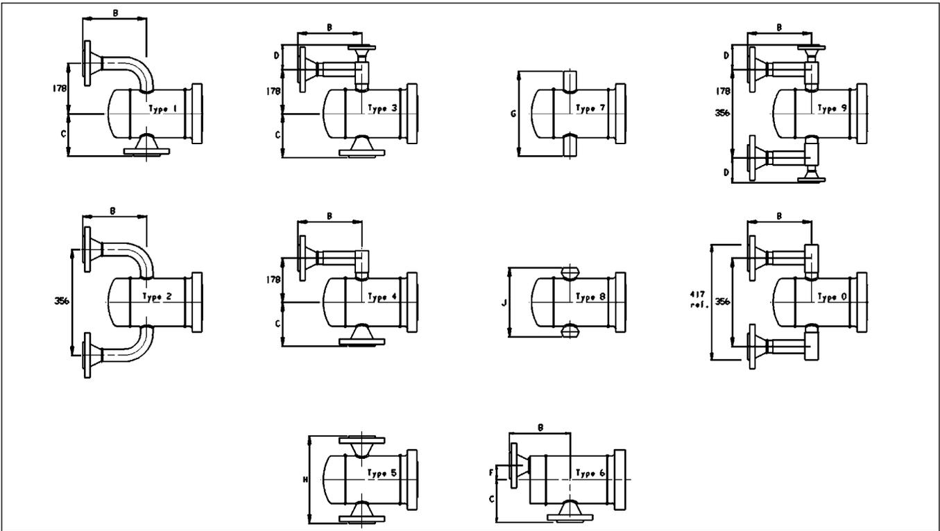
**Fabricated chambers** Standard dimensions: Ref. only - must be certified on order
