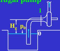
Near the center of impeller, the pressure  $p_1$  is lower than  $p_0$ , so that the liquid is sucked into the pump.
