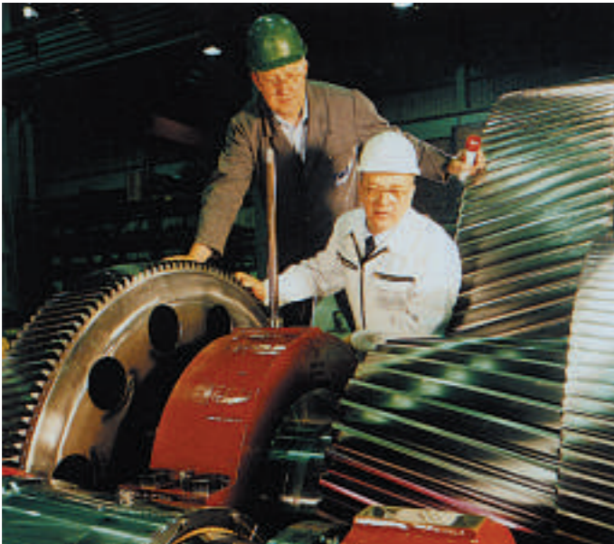
Inspection of a Marine Gear Box
