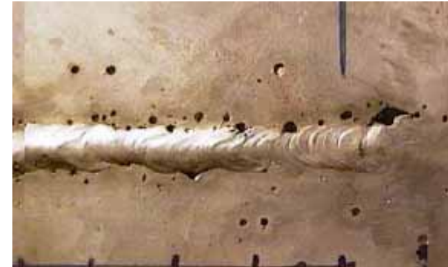
Pitting corrosion in stainless steel 不锈钢点腐蚀
