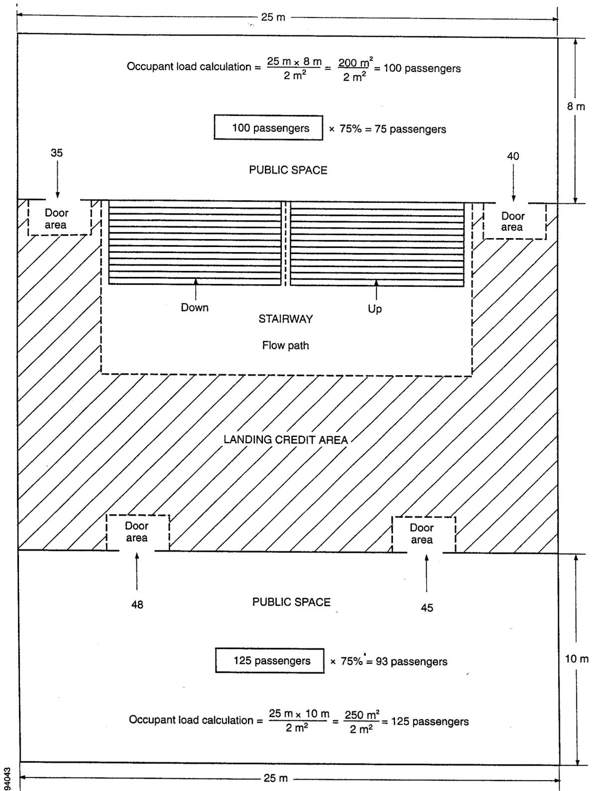
Figure 3 – Occupant loading calculation example
