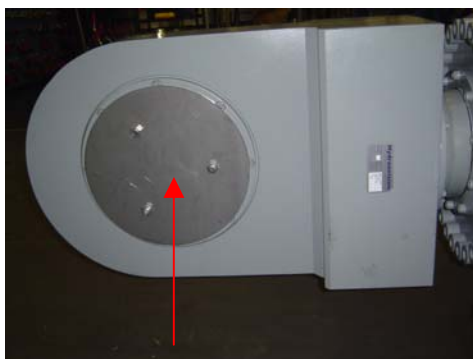
Protection cover on ball bearing
