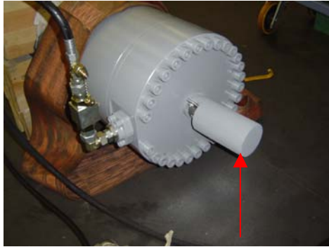
Protection cover on electric connections
