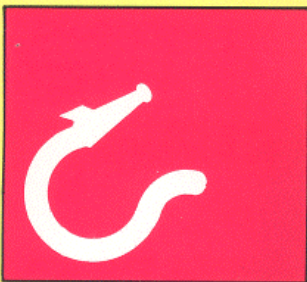
Hose box with spray/jet fire nozzle
