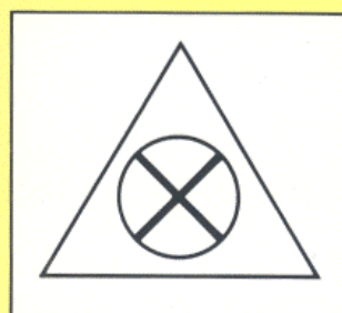
Remote ventilation shutoff
