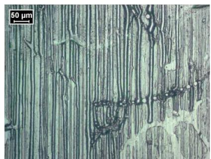
Fig.1 Unit #5 - top ring, particles in running surface (713X)
