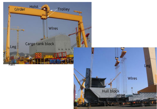
Fig. 1 Example of a gantry crane for lifting ship erection blocks
