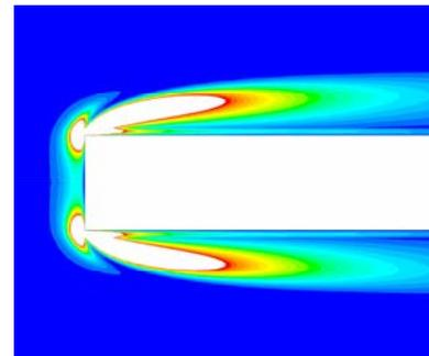
The Standard k-ε model is known to give spuriously large TKE on the front face of the plate
