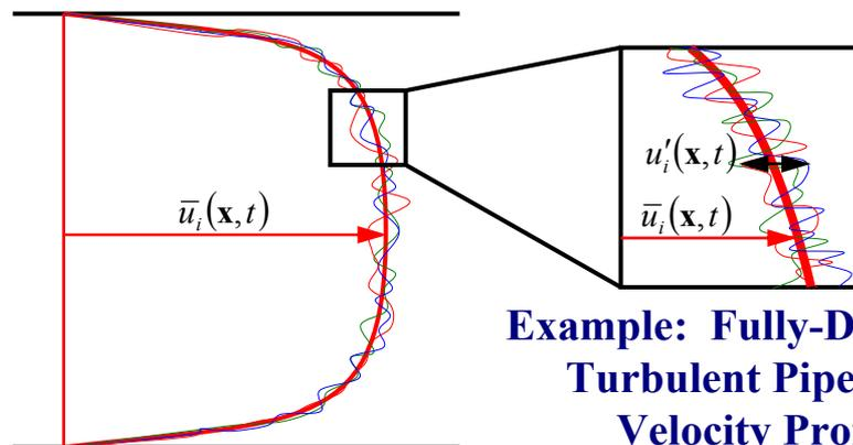
**Example: Fully-Developed Turbulent Pipe Flow Velocity Profile**
