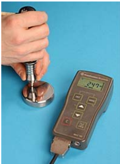
Fig.3. Ultrasonic testing using a Microdur unit
